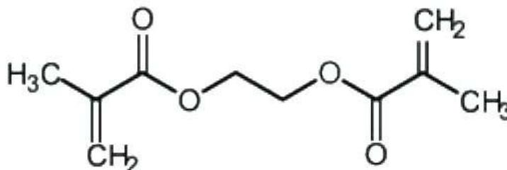
Ethyleneglycol dimethacrylate, EGDMA acts as a cross-linking agent between polymer chains. Also known as ethylene dimethacrylate or monoethylene glycol dimethacrylate, this difunctional monomer has similar reactivity to methyl methacrylate and low water absorption.
